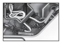
C5. Use the remaining included zip ties (6) to secure the harness to the chassis (refer to Fig. 2 Chassis Wiring for more detail).
